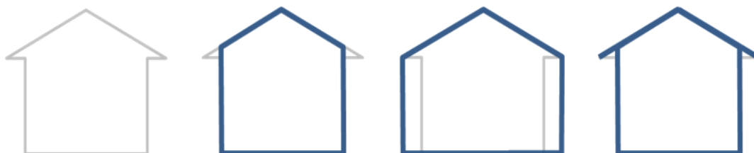
Figure 11: From left to right: a BuildingPart with a roof overhang in light grey, a BuildingPart modelled by working from the BGT, a BuildingPart modelled by working from the BAG and a BuildingPart modelled by working from both the BGT and the BAG.
