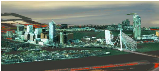
3D City model from laser point data, by IT-Pro-People (with Bentley software Terra Solid)
