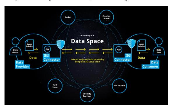
Figure 3.2 — IDS building blocks for data exchange (source: <u>IDSA infographic</u>)
